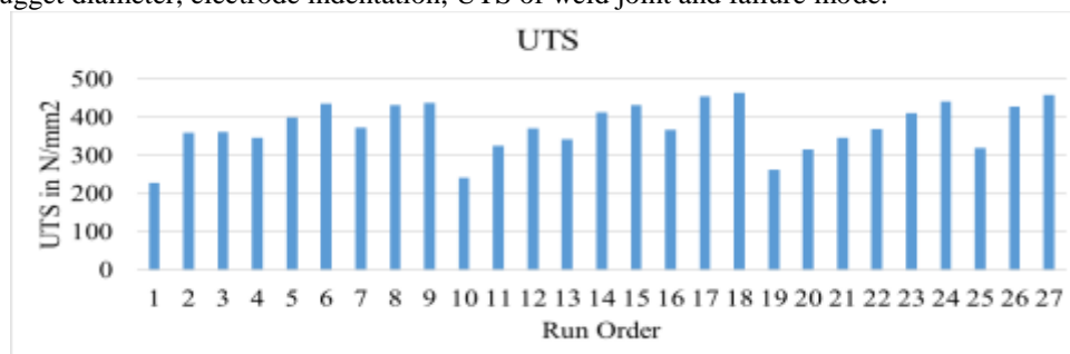
Fig. 2 Graphs on output of DOE for dissimilar spot welding of DP600 with AISI 304L
